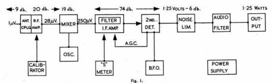
Block diagram of the receiver discussed in the text, showing approximate gains (db.) per stage and indicating the voltages appearing at various stages when a 1  $\mu$ V. signal is applied to the aerial terminals.
