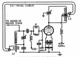
Fig. 1. Stabilising the 813 Valve.
