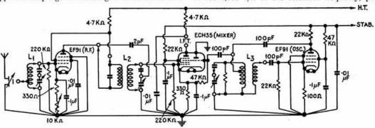
Fig. 2. R.F., mixer and oscillator circuit.
