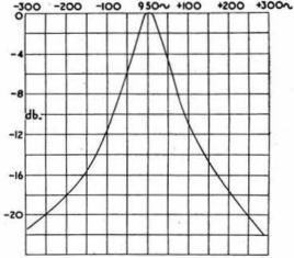
Fig. 5. Audio Filter response curve.
