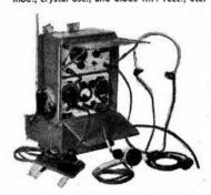
Receiver, superhet circuit, employing 6 valves, ILN5 H.F. Amp., ILA6 Ist det. F.C., ILN5 I.F. Amp., ILD5 2nd det. and B.F.O., ILD5 1st L.F. and A.V.C., IAS output, I.F. frequency 455 kc/s., etc. Hand Driven Generator, supplying H.T. and L.T. (plus 12 V. bias, when switched for WS-18), with operator's seat.
